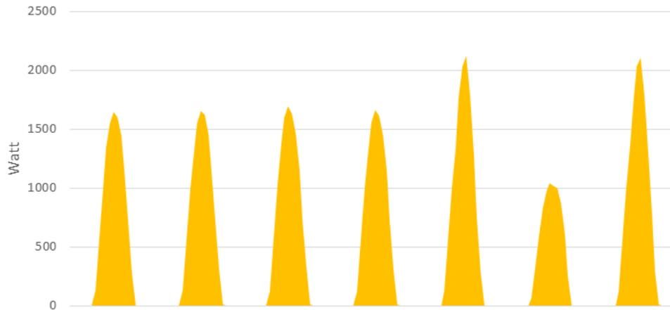
Figure 6 Representative solar profile AC System Output (W) - January 1 -7
