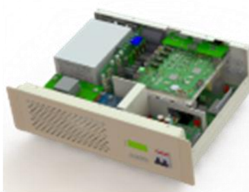
Battery Inverter 5kW
