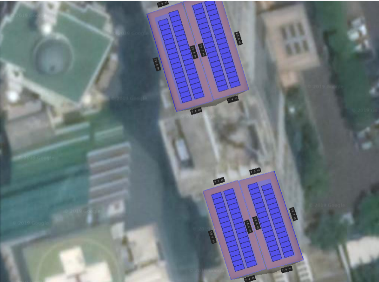
Snapshot (example of panel arrangement on top of Dinas Kesehatan DKI Jakarta building)
