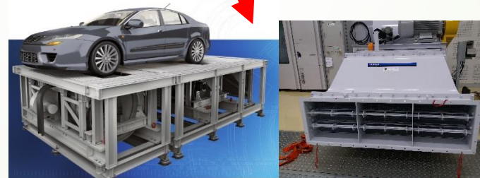
Road Simulation (CHASSIS DYNO & COOLING FAN)
