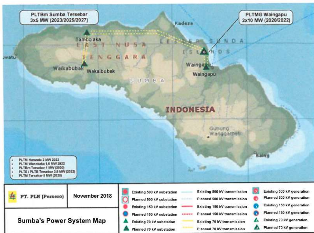
Figure 13. Sumba Island's power system map. Adapted from PLN's 2019 RUPTL
