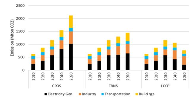
**Figure 14.** Projection of energy sector emissions by emitting sector under CPOS, TRNS and LCCP
