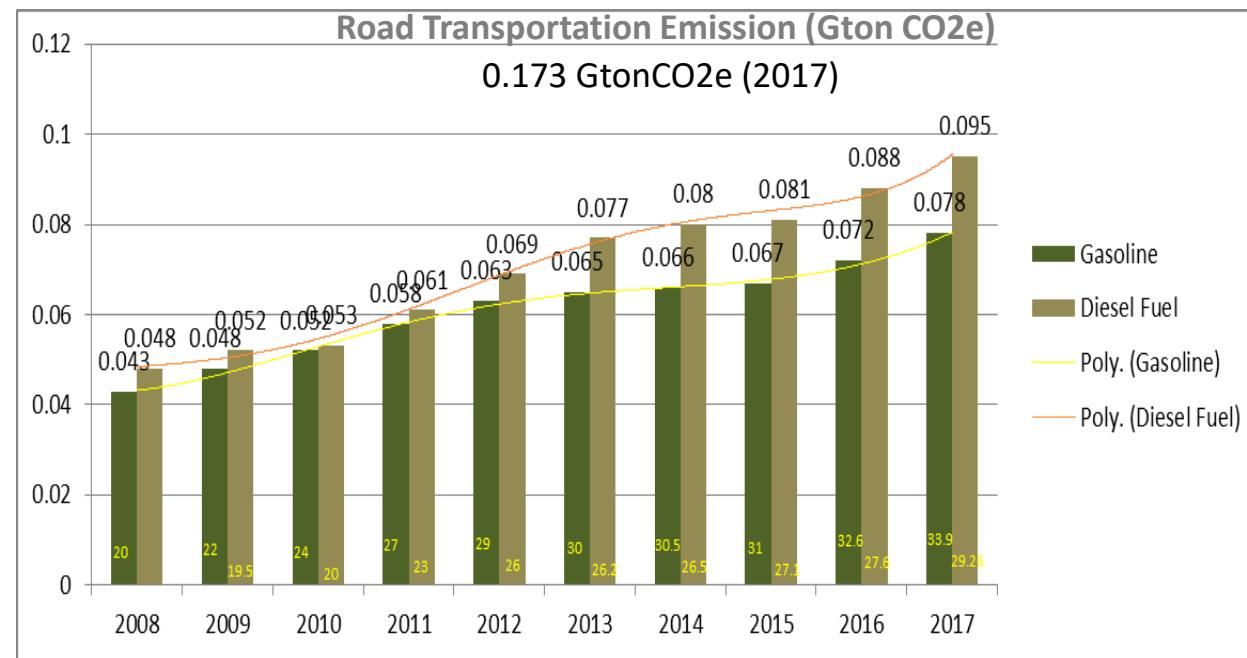
Road transportation consumed 63.1 million KL of fuels and emitted 173 MtonCO<sub>2</sub>e (2017), 255 MtonCO<sub>2</sub>e (2019), and tend to increase to be 470 MtonCO<sub>2</sub>e BAU (2030) (16.66% Nat'l GHG BAU).
