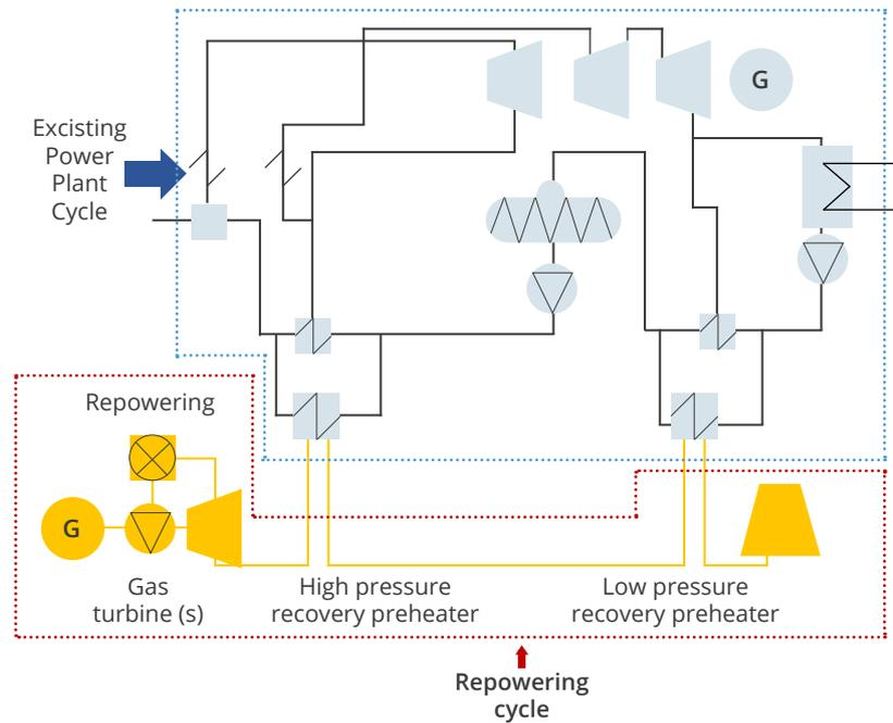
Figure 6. Diagram of repowering cycle in CFPP (Agora Energiewiende, 2017)
