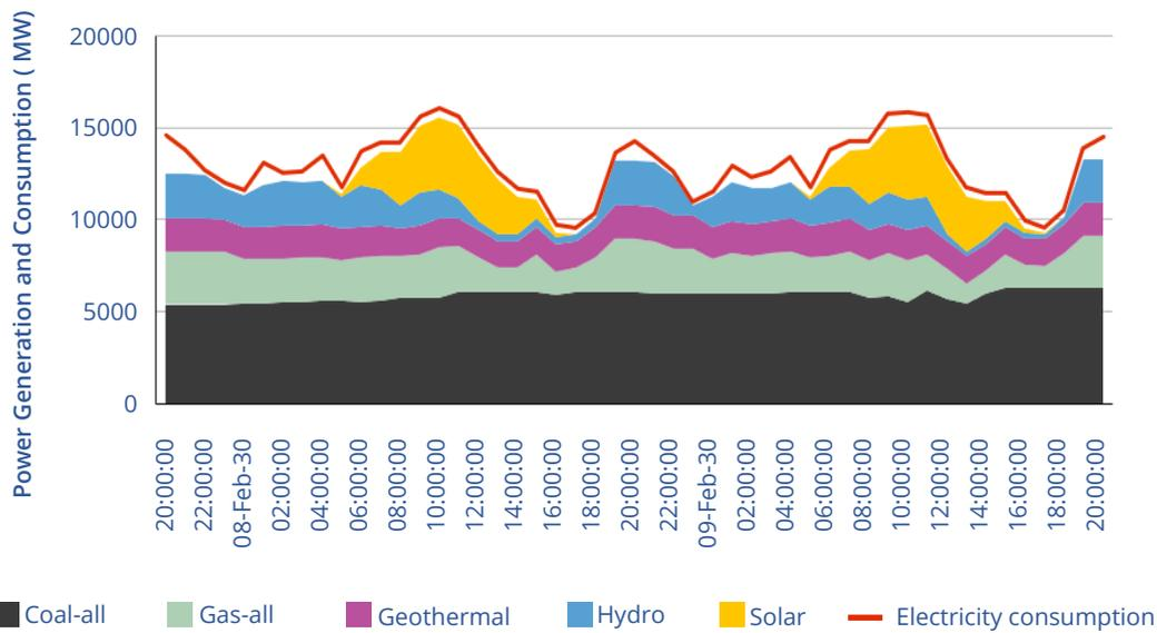
Figure 23. Power generation from CFPPs, GFPPs and renewable plants (solar PV, hydro and geothermal) and consumption within Sumatra system during low solar irradiation in 2030
