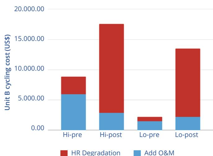
Figure 35. Unit B cycling cost breakdown
