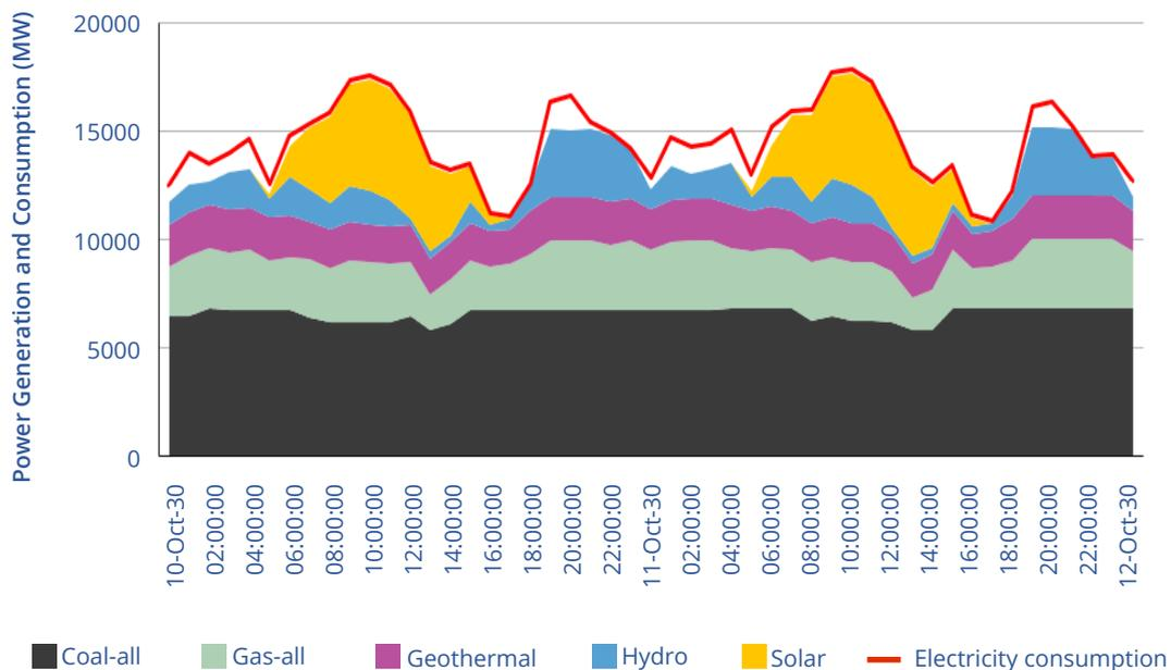
Figure 22. Power generation from CFPPs, GFPPs and renewable plants (solar PV, hydro and geothermal) and consumption within Sumatra system during high solar irradiation in 2030
