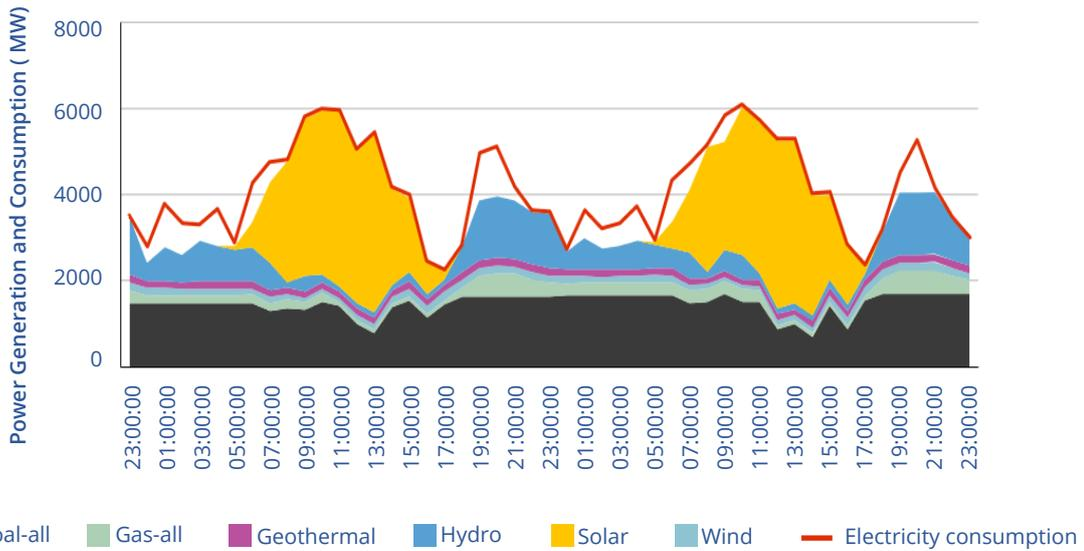
**Figure 28.** Power generation from CFPPs, GFPPs and solar PV plants and consumption within Sulawesi system during high solar irradiation in 2030
