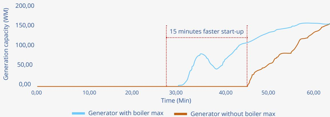
**Figure 8.** Improvement in the start-up time using BoilerMax (Agora Energiewiende, 2017)
