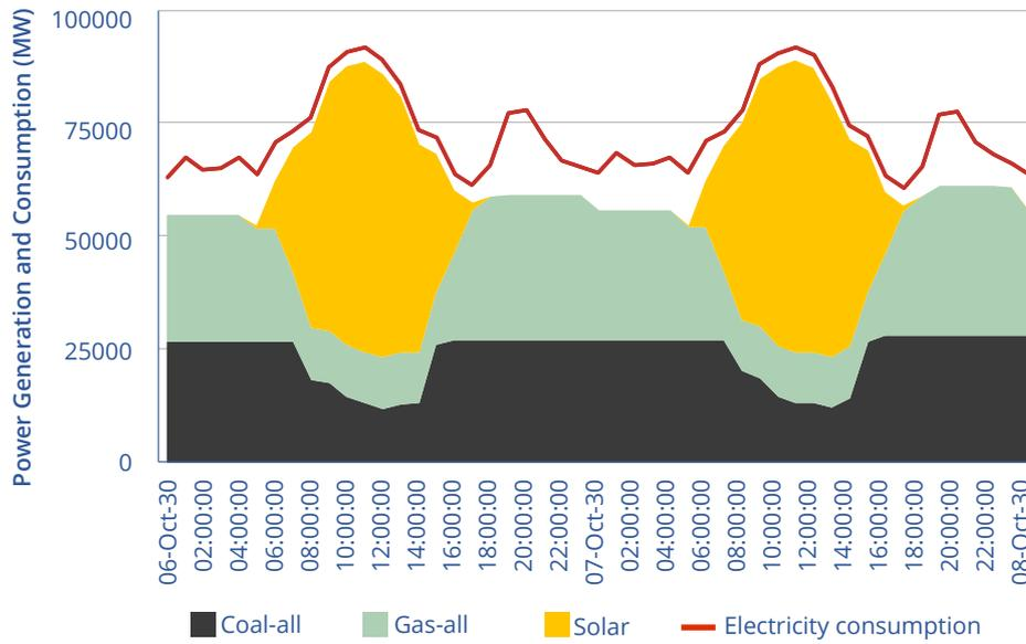
**Figure 25.** Power generation from CFPPs, GFPPs and solar PV plants and consumption within Java-Bali system during high solar irradiation in 2030
