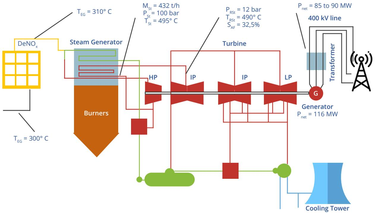
Figure 9. Operational parameters for the new load operation in Bexbach power plant (Heinzel et al., 2012)
