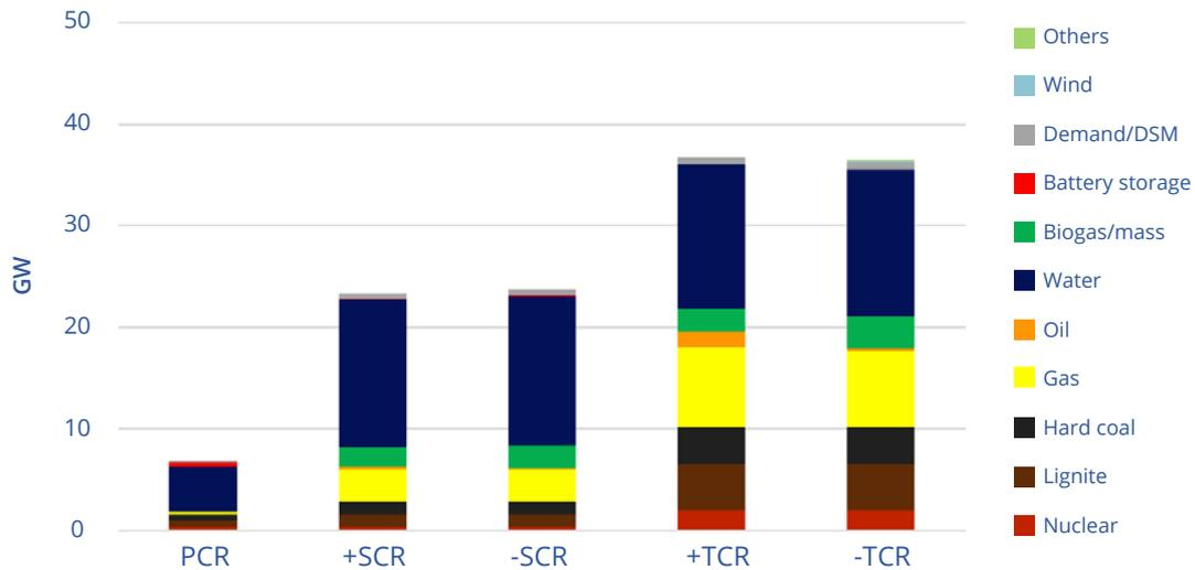
Figure 14. Prequalified balancing capacity (in GW) in Germany from various primary energy source (Consentec, 2020)
