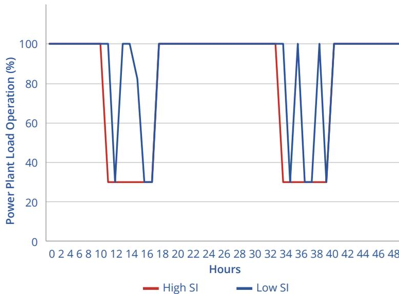
Figure 27. Typical 600 MW CFPP load operation in Java-Bali system during high (High SI) and low (Low SI) solar irradiances
