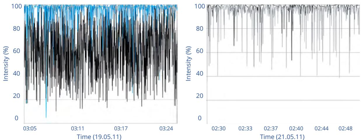
Figure 11. Comparison of the two mills (left) and single mil (right) I operation in Heilbronn unit 7 trial run
