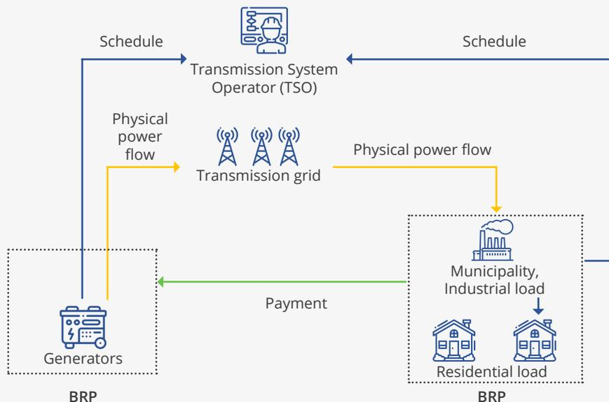
Figure 12. Illustration of the balancing mechanism in Germany (Ernst, 2015)
