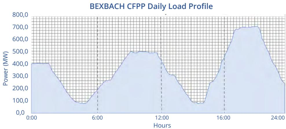
Figure 10. Typical daily load profiles operating at full and minimum loads (Heinzel et al., 2012)
