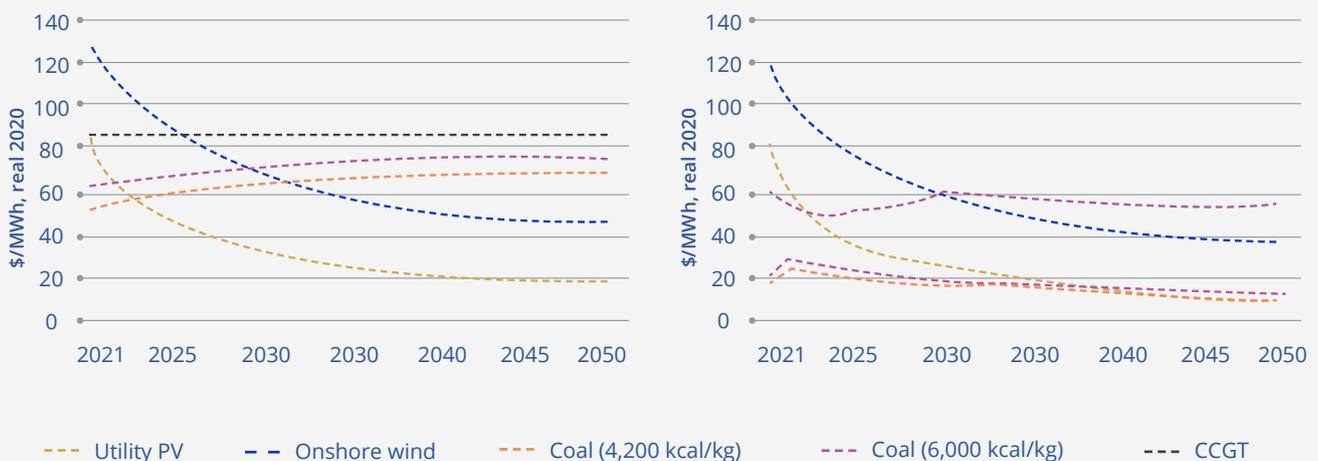
Figure 3. LCOE comparisons of utility PV (solar) and onshore wind, respectively, to new CFPP (left), and short-run marginal costs for CFPP (right) (BNEF & IESR, 2021)
