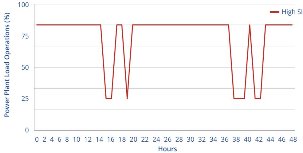
Figure 30. Typical 100 MW CFPP load operation in Sulawesi system at high (High SI) solar irradiance
