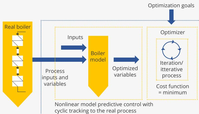
Figure 7. Principle mechanism of BoilerMax (ABB Group, 2014)
