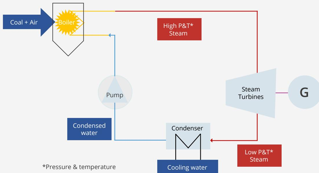
Figure 5. Simple illustration of a CFPP working principle
