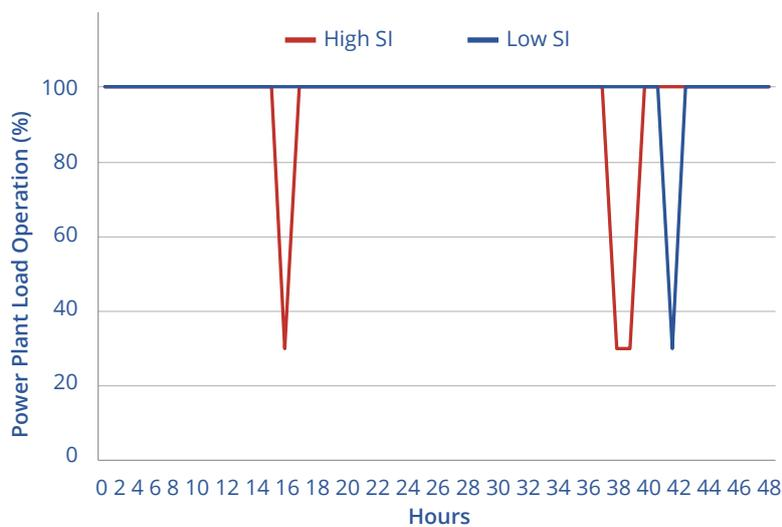
Figure 24. Typical 100 MW CFPP load operation in Sumatra system during high (High SI) and low (Low SI) solar irradiances
