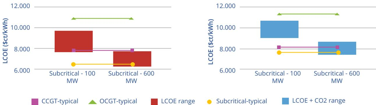
**Figure 37.** Flexible CFPP LCOE estimation for two subcritical units with different capacity class, i.e. 100 MW and 600 MW: **top** - LCOE, **bottom** - LCOE with CO<sub>2</sub> price
