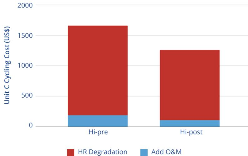
Figure 36. Unit C cycling cost breakdown
