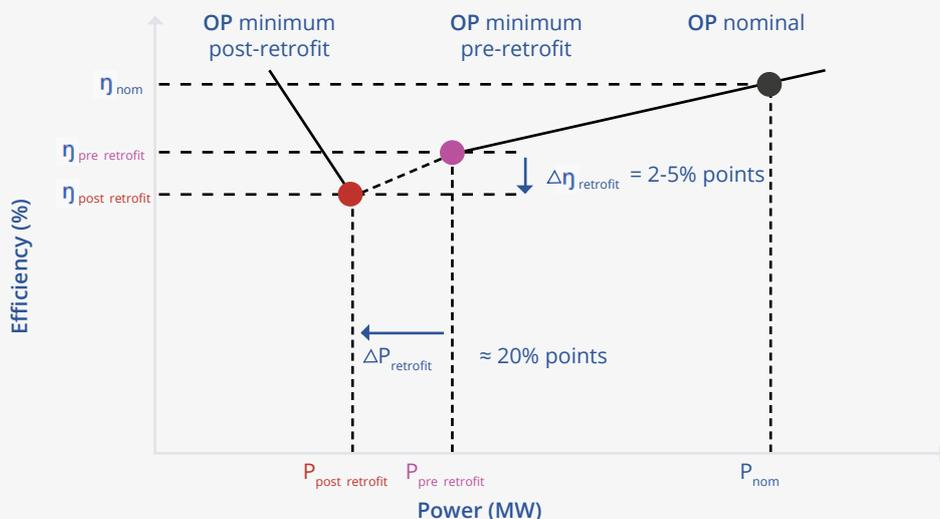
Figure 21. Reduction in the efficiency as the result of lowering CFPP minimum load (Agora Energiewende, 2017)
