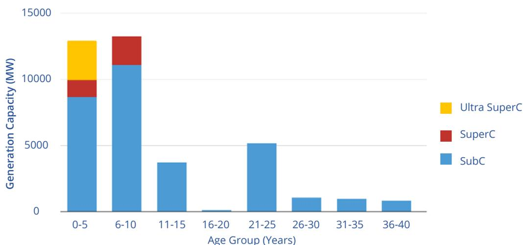
Figure 20. Steam cycle technology utilised in Indonesia's CFPP unit
