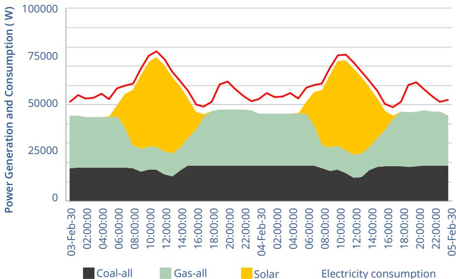
**Figure 26.** Power generation from CFPPs, GFPPs and solar PV plants and consumption within Java-Bali system during low solar irradiation in 2030
