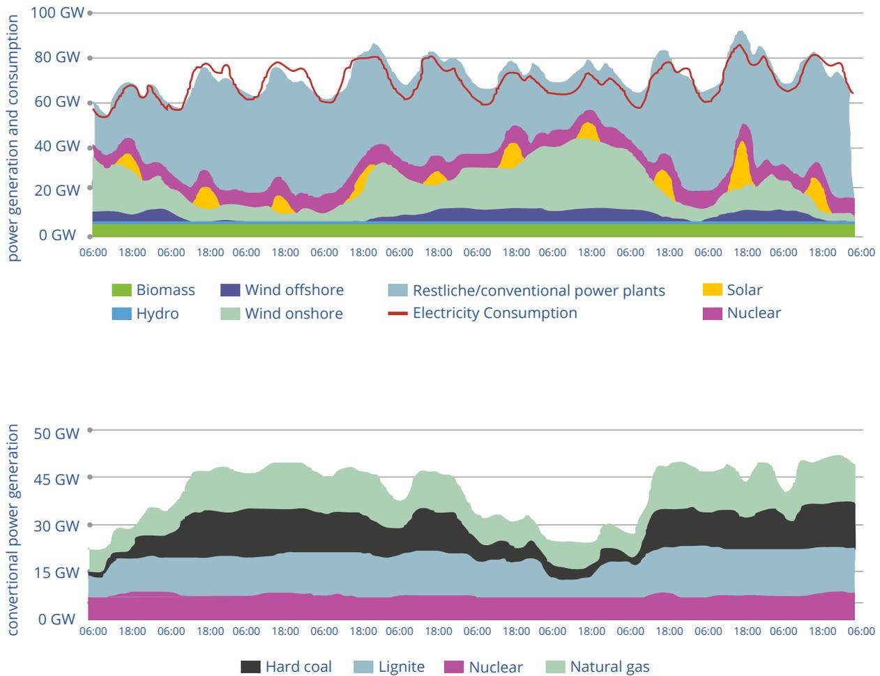
**Figure 5.** Upper power generation of all power plants (including the renewables) and consumption profiles in Germany during 10 days in November 2021; Lower breakdown on the conventional power plants generation within the same period of time (Agora Energiewende, n.d.)
