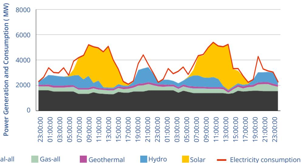
**Figure 29.** Power generation from CFPPs, GFPPs and solar PV plants and consumption within Sulawesi system during low solar irradiation in 2030
