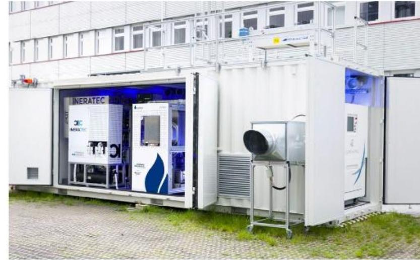
applications. The project, called C2 Fuels is deploying a small solid oxide system, with electrical capacity in the single-digit kW, in Dunkirk, France.<sup>49</sup>
